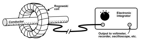
the integration parameters the sensitivity of the complete measuring system, measured in Amperes per Volt, can be varied over about five orders of magnitude. The output from the integrator can be used with any form of electronic indicating device such as a voltmeter, oscilloscope, protection system or metering equipment.
